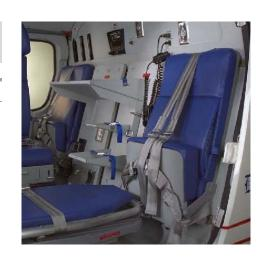
The seat design is installed with, four-point inertial restraint system, adjustable backrest and can easily be installed or folded away as seating needs require.
