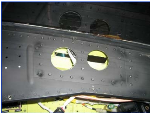
POSITION DOUBLER AS SHOWN, JUST BELOW HOLES ON UPPER SKIN.
