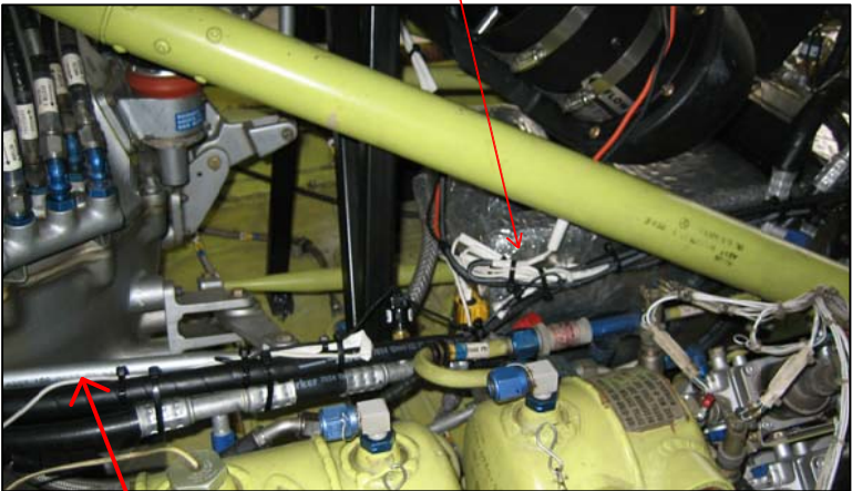
COMPRESSOR WIRE RUNS AFT. WITH FREON LINES TO COMPRESSOR
