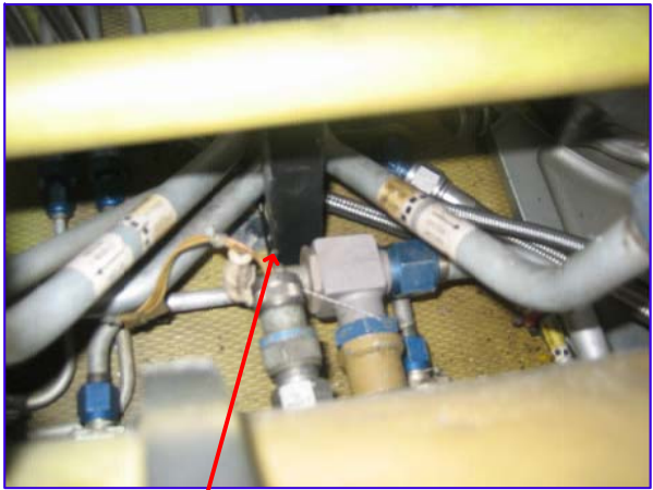
RIGHT/AFT CONDENSER SUPPORT FOOT LOCATION. INSTALL AN3-13A
